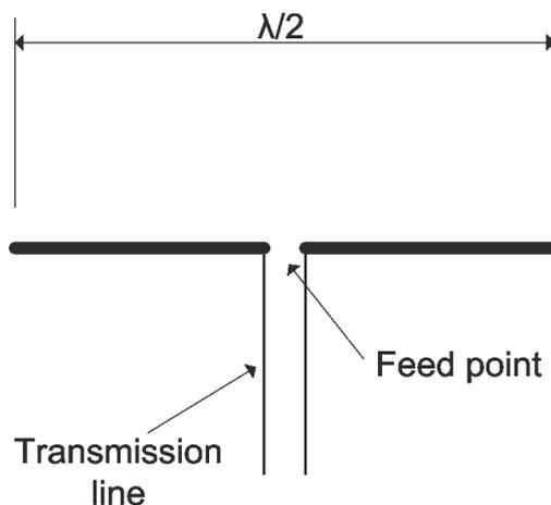
**Figure 3-9 The half wave dipole antenna showing a balanced transmission line feed at the mid-point**
