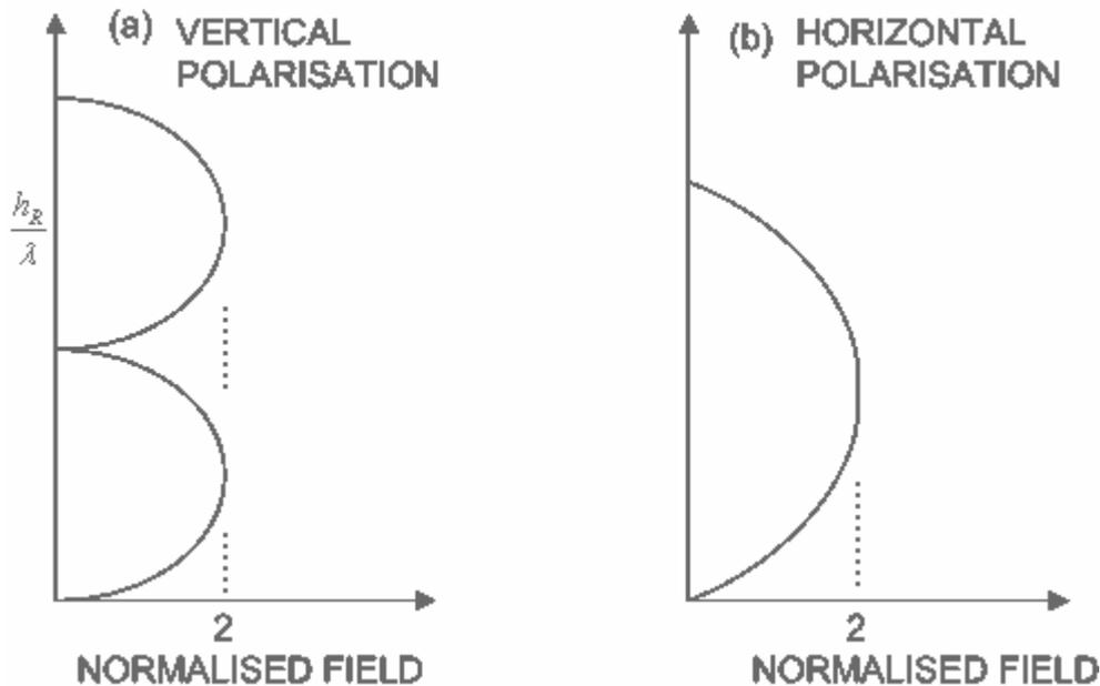
**Figure 3-3 Received field strength against receiving antenna height**
