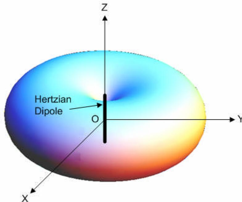
**Figure 2-2 The three dimensional shape of the radiation pattern of a Hertzian dipole which is aligned with the  $z$  axis, positioned with its mid-point at  $z = 0$**
