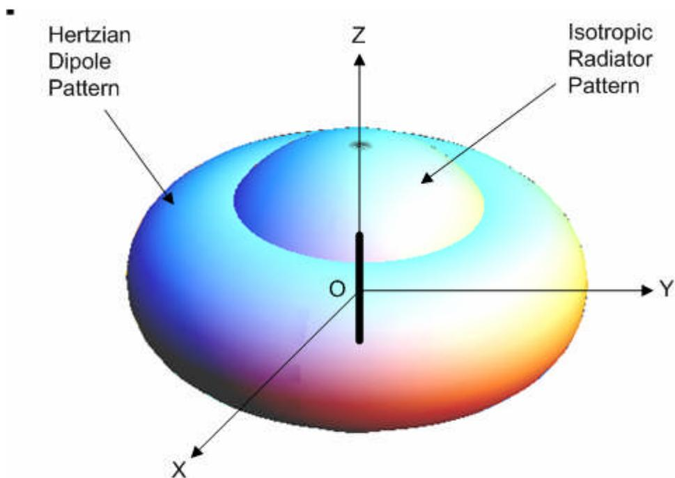
**Figure 2-5 The three dimensional radiation patterns for a Hertzian dipole and an isotropic radiator to the same scales**
