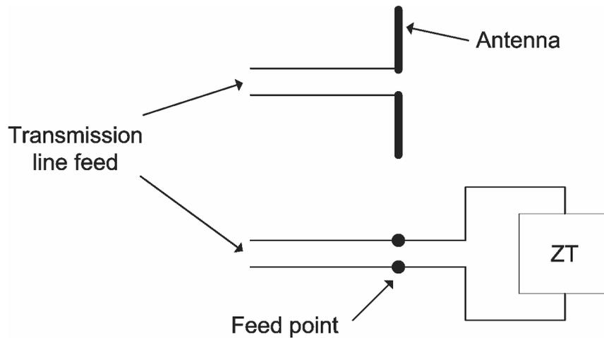
**Figure 3-8 An antenna showing connection of the equivalent feed point impedance  $Z_T$**
