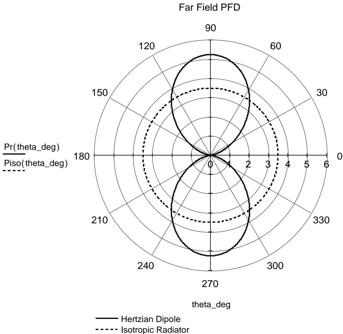
**Figure 2-4 Combined far field radiation pattern plots in two dimensions for the Hertzian dipole and the isotropic radiator for the example in Section 2.5. The radial scaling is the PFD expressed in picowatts per square metre (pW/m<sup>2</sup>)**
