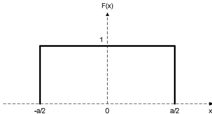
**Figure 3-11 A uniform aperture illumination of  $1 \text{ V/m}$  in one dimension**
