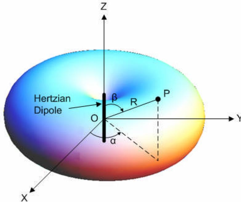
**Figure 2-3 An arbitrary point P on the surface of the radiation pattern which is represented in spherical co-ordinates by  $(R, \alpha, \beta)$**
