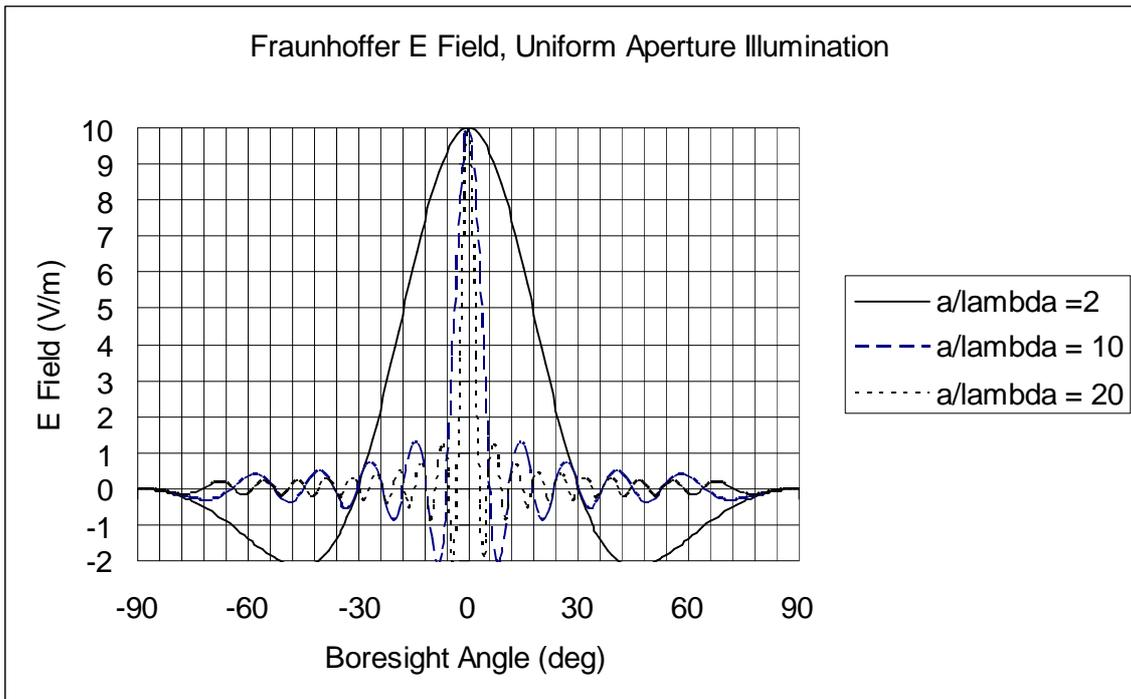
**Figure 3-12 One dimensional Fraunhofer radiation pattern for uniform aperture illumination, for three values of  $a/\lambda$**
