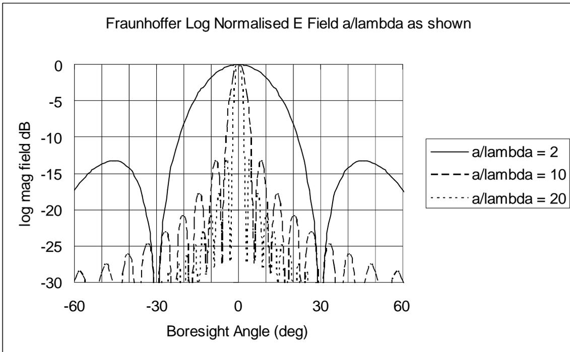
**Figure 3-13 The one dimensional Fraunhofer radiation pattern represented in normalised logarithmic form for uniform aperture illumination**
