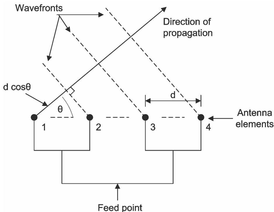
**Figure 5-1 A schematic of the broadside linear array with all elements fed in phase**
